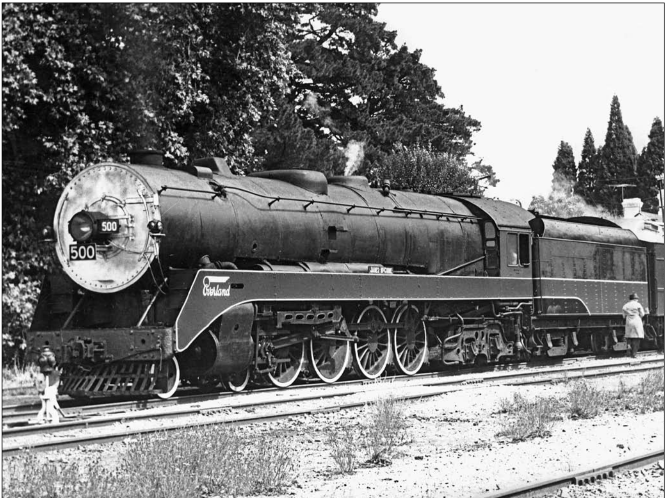
Below: Number 500 on an ARHS tour at Mount Barker on 17 March 1963. It has been repainted in the green and black livery. It now features a front end throttle on the rear of the smokebox. It is not known if any other 500s received this modification. Photo: National Railway Museum collection BU08902.
