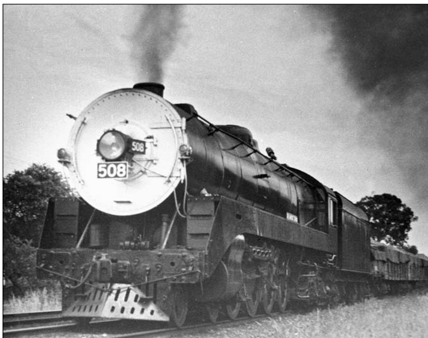
Above: 508 has also got a pressed steel pilot/cowcatcher as it heads a freight out of town. Photo: National Railway Museum collection BU21038.
